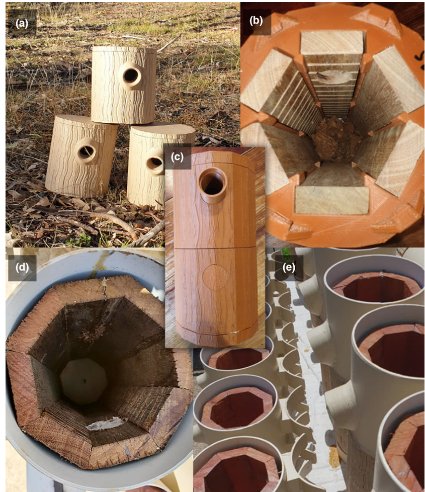
FIGURE 1 Different designs of plastic nest boxes compared in climatic trials. (a) Nest box Type 1: 3D-printed nest box, with no timber inserts. Note the textured bark exterior. (b) Nest box Type 2: Double-height, 3D-printed nest box with timber inserts (unpainted). The air space between the double walls has been enclosed in the design and is not visible; decomposed heartwood timber furnishes the base. (c) Double-height, 3D-printed nest box showing entrance, and blank that closes off the lower entrance hole; bayonet-style fittings allow for multiple body sections to be connected. (d) Nest box Type 3, with octagonal timber insert fitted inside a 150-mm diameter PVC pipe housing, showing marine plywood base with central drainage hole, drilled entrance hole and horizontal cuts in timber inserts to facilitate fauna egress. (e) A range of PVC/timber habitat hollows showing the octagonal hardwood timber insert, 3D-printed entrances, and bracket systems for fitting to trees, power poles and other convex structures
